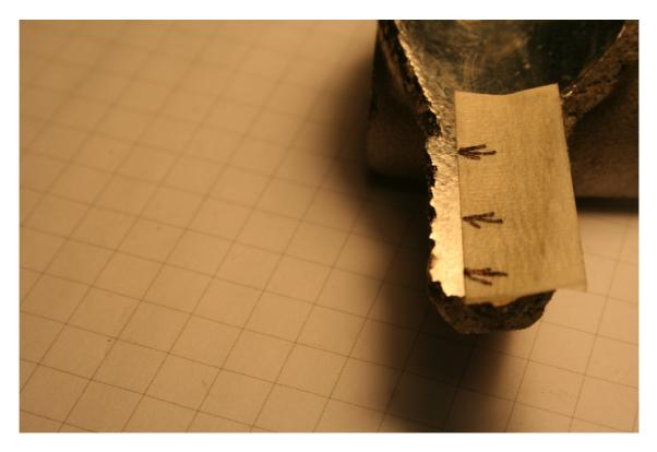
Figure 3 shows another section where these network cracks were present; location has been marked with arrows.
