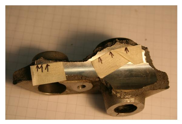
It was also noted that the external surfaces of the fork legs had been shot peened and a clear finish was present. A check with an ohm meter showed that the finish was non-conductive, which is characteristic of a paint type coating or anodizing. Scraping with a knife showed the coating to come off, which is consistent with a paint (clear coat) type of coating. Anodize would have resisted scraping.
