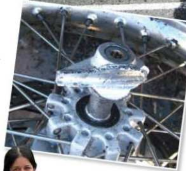
Rashmi Tambeh (below) lost control of her bike on a straight smooth road when the front wheel came adrift (above). The front axle mount casting had failed (left)
