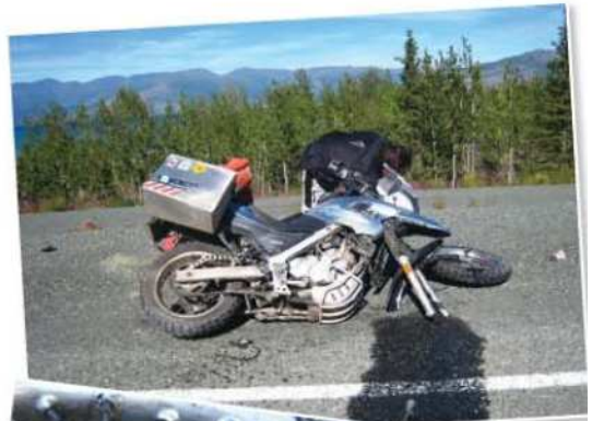
Rashmi Tambeh (below) lost control of her bike on a straight smooth road when the front wheel came adrift (above). The front axle mount casting had failed (left)
